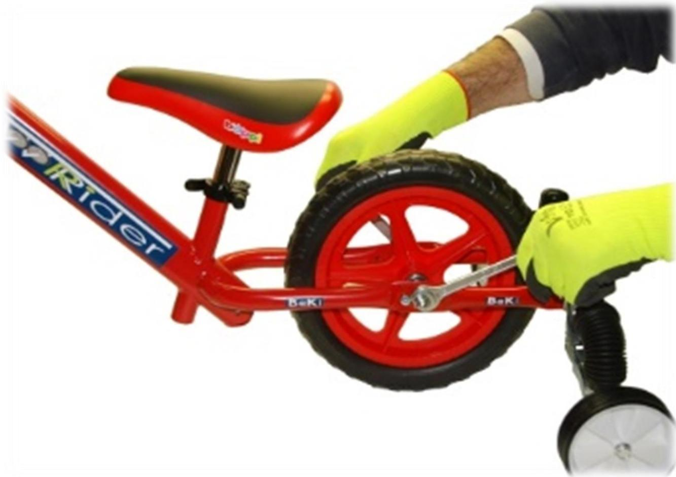
TIRARE BENE I DUE DADI E LE DUE VITI A CROCE. IL SELLINO ALL'INIZIO NON VA SERRATO TOTALMENTE, MA SOLO A SUFFICIENZA PER RENDERLO STABILE. PER ABBASSARLO AL MINIMO VA SPINTO CON FORZA VERSO IL BASSO, CON LA LEVA SERRATA. PER REGOLARLO, AL MOMENTO DI RIALZARLO, VA TIRATO VERSO L'ALTO PER SCOPRIRE LA LEVA DI SERRAGGIO E POTERLA MANOVRARE.
