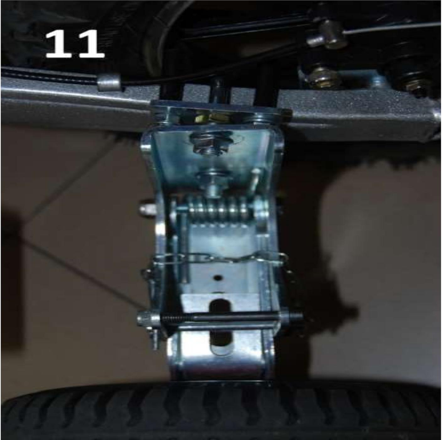
INSTALL A DESTABILIZER ON THE MOTORCYCLE (11). WITH CHILDREN ON BOARD AND MOTORCYCLE WALKING TO CHECK THE FLOOR THAT THE WHEEL OF THE TRANSPORTER PIPES TO EARTH PERPENDICULAR OR SLIGHTLY INCLINED NEXT TO THE PEDAL. IF THE RESULT IS OPTIMAL, PRACTICE THE HOLES ON THE SECOND COUPLE BY COUPLING IN A MIRROR
